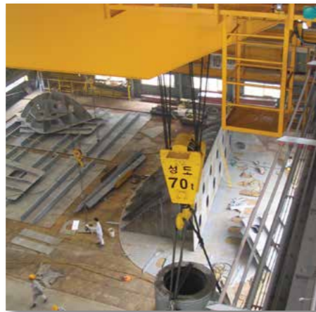
Double Overhead Hoist Crane
