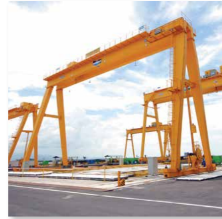
Gantry Hoist Crane
