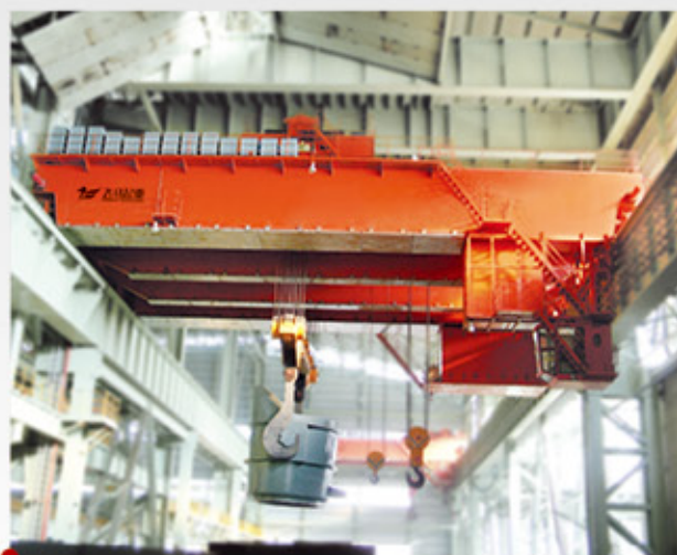
铸造桥式起重机 Casting bridge crane
