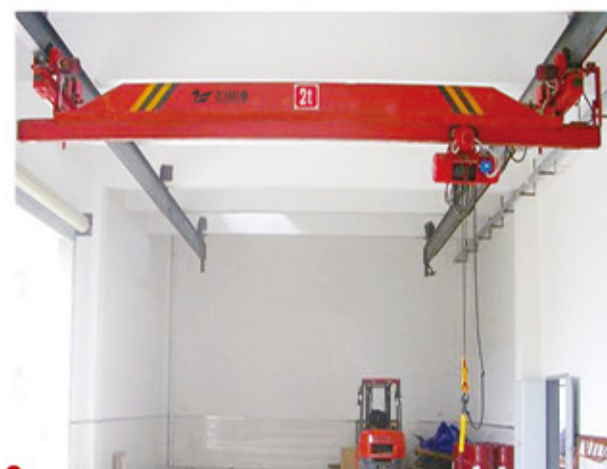
LX型电动单梁悬挂起重机 LX electric single beam suspension crane
