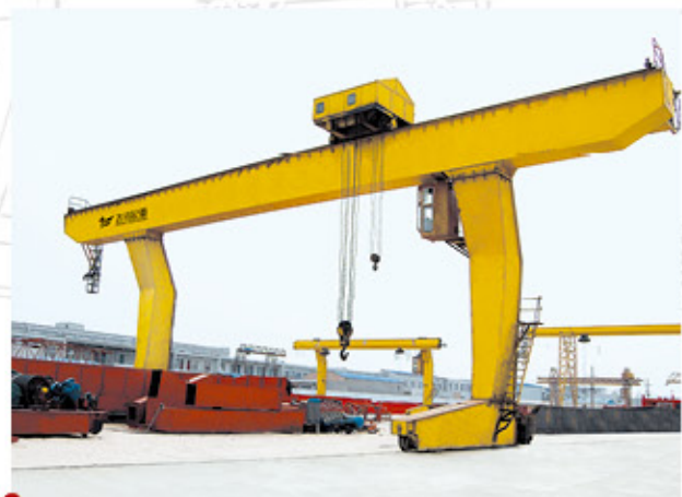
MDG型单梁通用门式起重机 MDG single beam universal gantry crane
